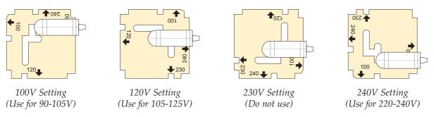
Mains Inlet Voltage Setting PCB
